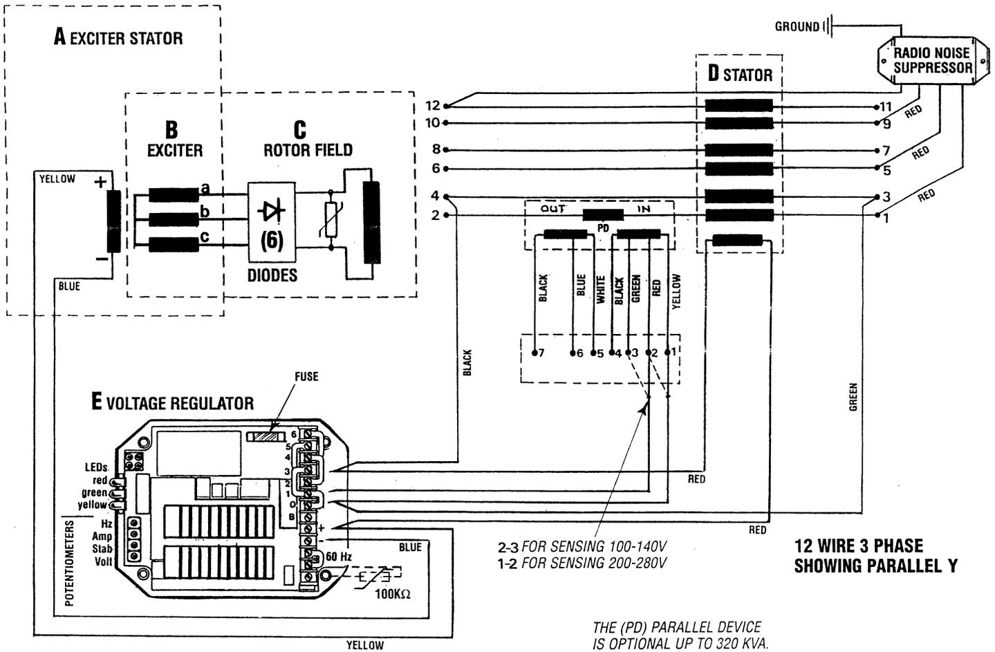
THE (PD) PARALLEL DEVICE IS OPTIONAL UP TO 320 KVA. THE LINK P ACTIVATES OR DE-ACTIVATES THE PARALLELING DEVICE IF IT IS PRESENT.
