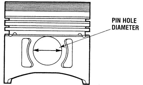
If an inside dial indicator is not available, use the following procedure to check the piston pin fit.
