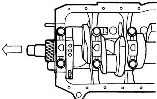
LUBRICATE CAP BOLTS WITH ENGINE OIL
