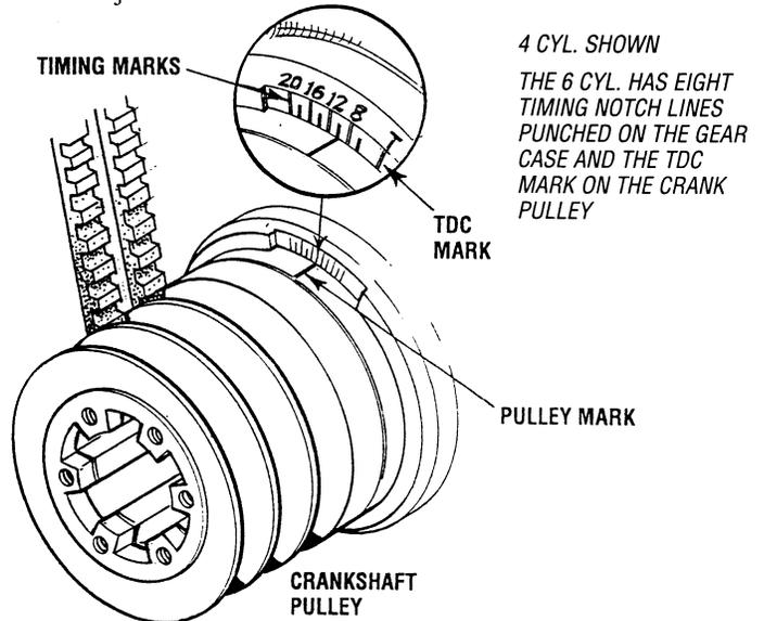
Check the crankshaft position for the start of fuel injection.
