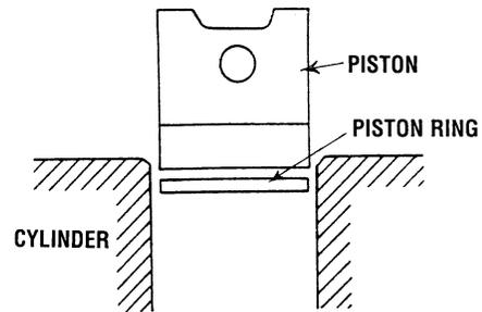
3. Use a feeler gauge to measure the piston ring gap.
