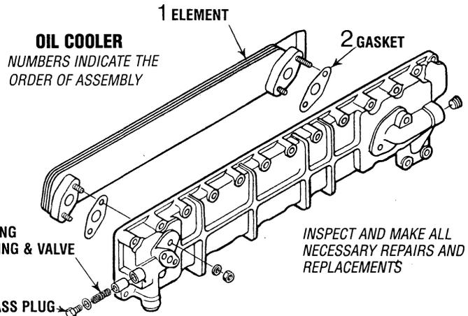
Install the oil cooler element to the oil cooler, and tighten the cooler element fixing nuts to the specified torque.
