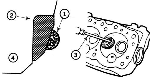
3. Use a screwdriver ③ to pry the valve seat insert free.
