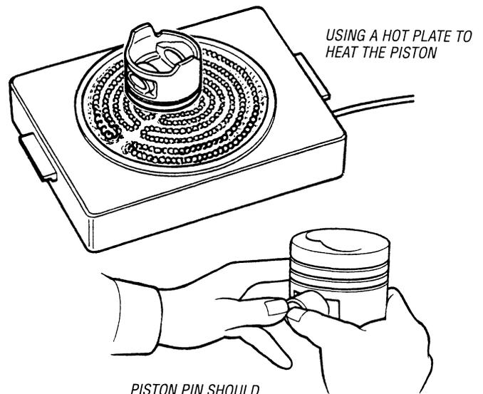
USING A HOT PLATE TO HEAT THE PISTON
