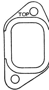
4 CYL. AND 6 CYL. USE DIFFERENT MANIFOLD GASKETS. 6 CYL. SHOWN
