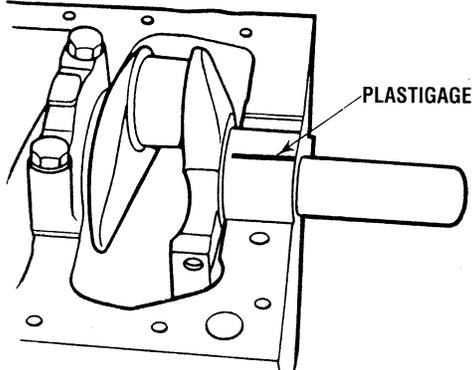
6. Install the bearing cap with the bearing.
