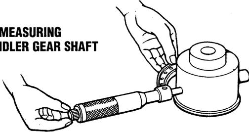
2. Use a dial indicator to measure the idler gear inside diameter.
