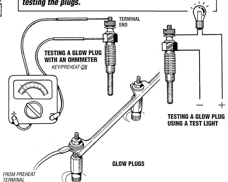
Re-install the plugs in the engine and test them again. The plugs should get very hot (at the terminal end) within 20 to 25 seconds. If the plugs don't heat up quickly, check for a short circuit. When reinstalling the glow plugs, use anti-seize compound on the threads.
