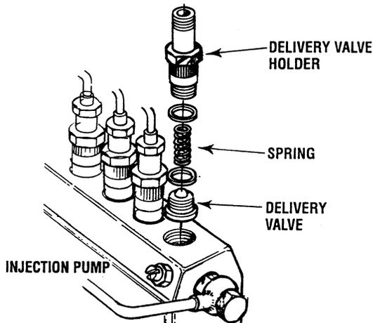
3. Remove the injection pump No. 1 delivery valve holder, delivery valve and spring and reinstall the delivery valve holder back into the pump.
