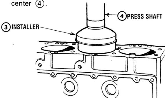
7. Check that the cylinder liner is set perpendicular to the cylinder.
