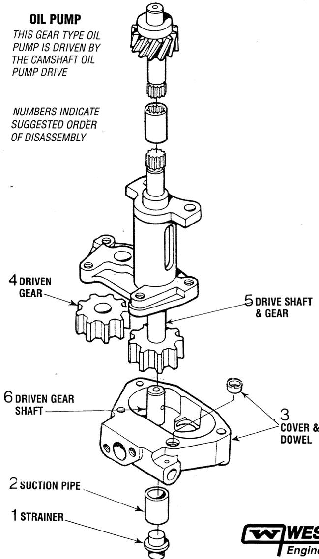
Visually inspect the disassembled parts for excessive wear and damage.
