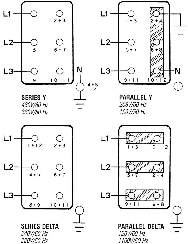
**NOTE:** IF WIRING FOR 50 Hz, THE 60 Hz JUMPER MUST BE REMOVED FROM THE REGULATOR.
