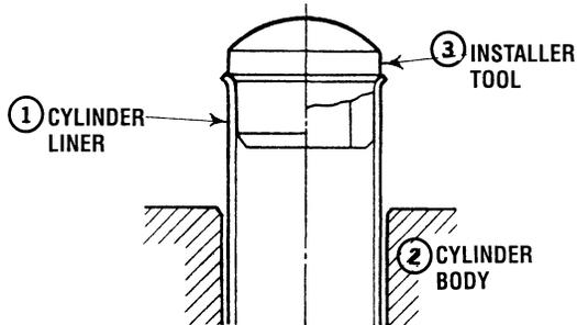
4. Insert the cylinder liner (1) into the cylinder body (2) from the top of the cylinder body.
