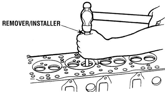
The height of the valve guide top edge from the cylinder head upper face should be 14.1 mm (0.55 in).
