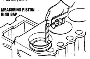
CLEARANCE BETWEEN THE ENDS OF THE PISTON RINGS
