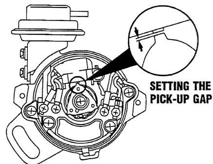
Adjust the point gap of the pick-up assembly between the rotor and the pick-up.
