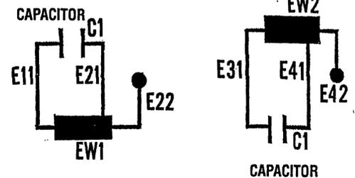
MAIN STATOR WINDING RESISTANCE LESS THAN ONE OHM FOR EACH WINDING GROUP
