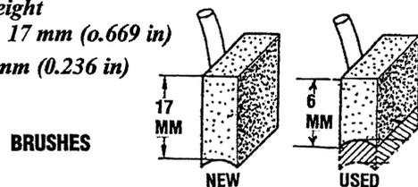
2. Check the brush spring tension. A weak or defective spring will cause excessive brush wear; replace the springs if suspect.
