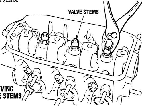
**REMOVING VALVE STEMS**
