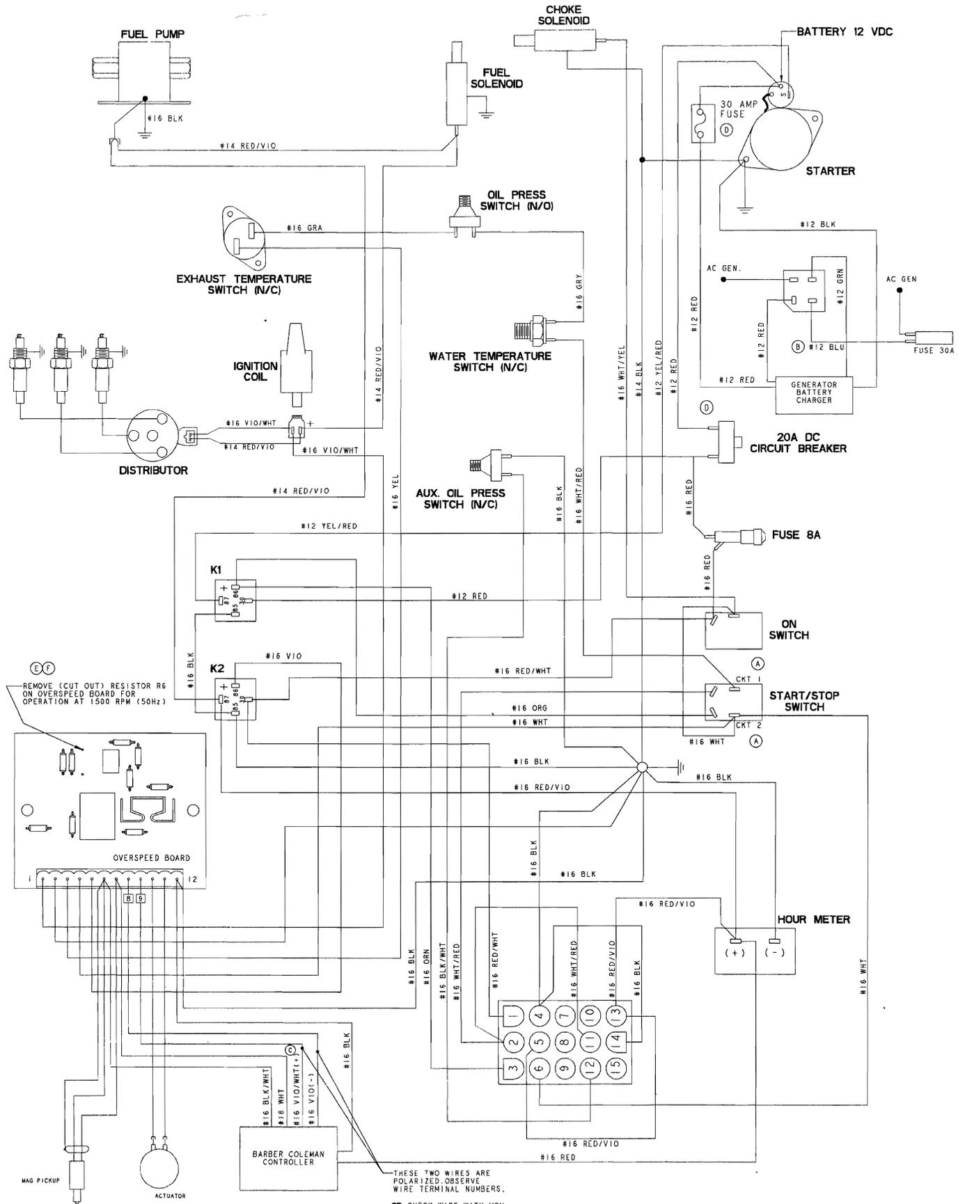
(E) REMOVE (CUT OUT) RESISTOR R6 ON OVERSPEED BOARD FOR OPERATION AT 1500 RPM (50Hz)
