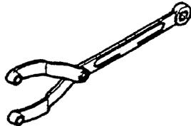
**CRANKSHAFT FRONT OIL SEAL INSTALLER**
