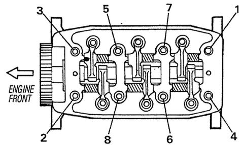
**CYLINDER HEAD BOLTS LOOSENING SEQUENCE**
