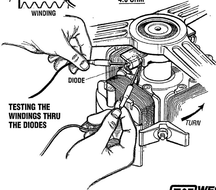
TESTING THE WINDINGS THRU THE DIODES
