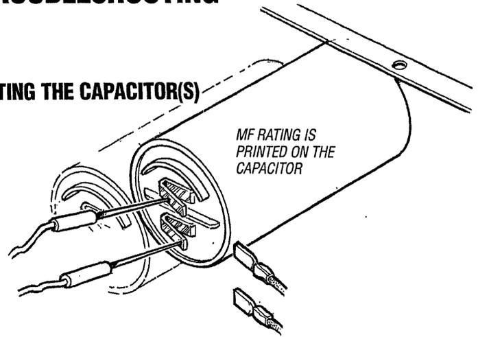
**⚠ WARNING:** *Capacitors must be discharged before handling as they store electricity and can pack a potentially lethal charge even when disconnected from their power source.*
