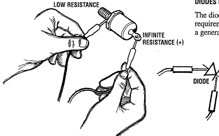
A low resistance should be found with the leads in one direction and infinite resistance (blocking) in the other direction.
