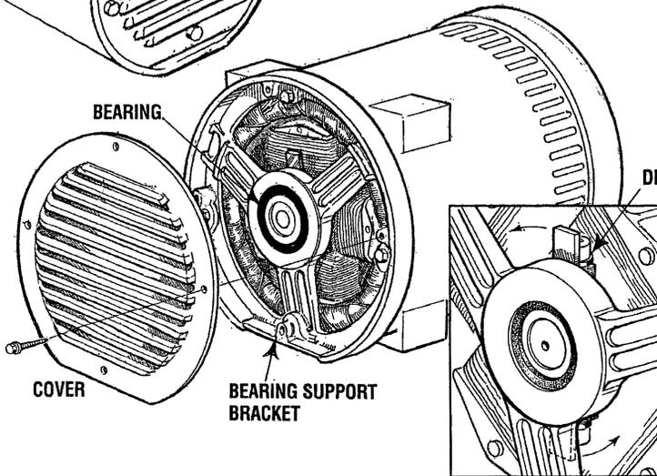
Testing the Mecc Alte generator can be accomplished without removing the bearing support bracket. Simply turn the armature to allow access for the testing as shown.
