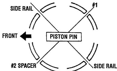
Insert the piston and connecting rod assembly into the cylinder, working from the arrow mark on the piston top toward the camshaft sprocket side.
