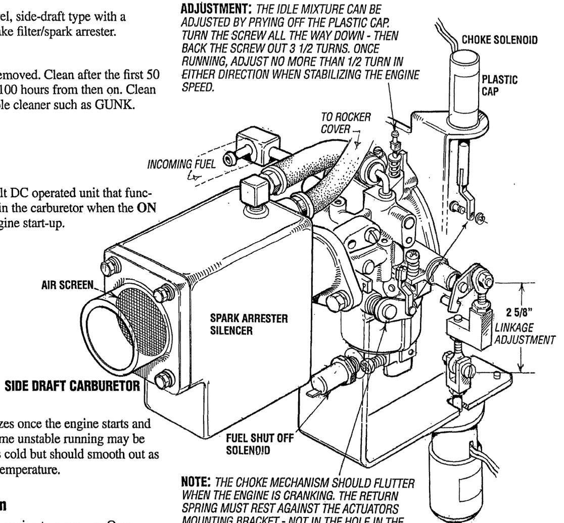
The choke solenoid de-energizes once the engine starts and the ON switch is released. Some unstable running may be present when the engine starts cold but should smooth out as the engine reaches operating temperature.
