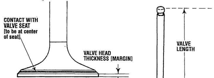
VALVE LENGTH: Intake 3.60in (100.6mm)
