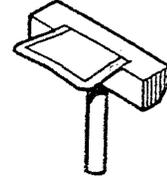
**CRANKSHAFT REAR OIL SEAL INSTALLER**
