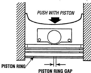
Check the piston ring for damage, wear, seizure and bends replacing the rings if anything unusual is noted. Always replace the piston rings when installing a new piston.
