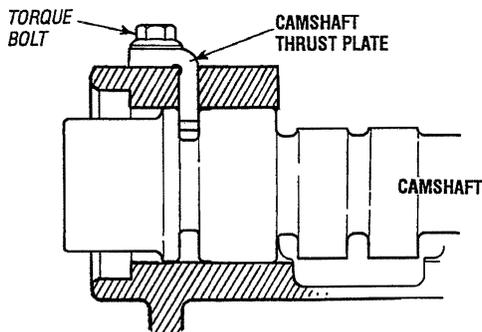
3. Measure the end play of the camshaft by inserting a feeler gauge in the gap between the rear of the thrust plate and the new front camshaft journal.
