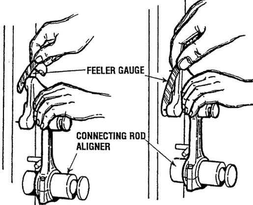
**CONNECTING ROD TWIST LIMIT** 0.004in (0.1mm)
