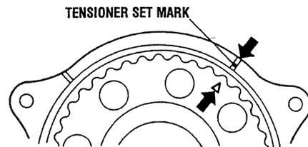
9. Make sure that the timing belt teeth are engaged with the camshaft sprocket teeth along the portion of the sprocket shown by the curved arrow in the illustration below. Then tighten the tensioner nut.
