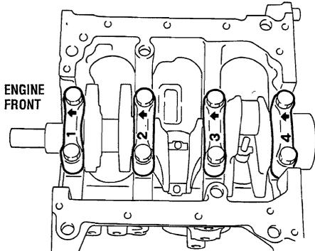
2. Install the bearing cap paying careful attention to the cap number and the arrow mark. Apply oil to the bolt threads.
