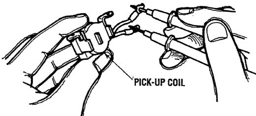
Check that when a screwdriver is passed near the iron core of the pick-up assembly the needle of the tester deflects.
