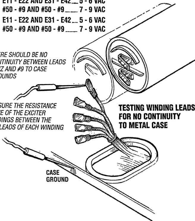
TESTING WINDING LEADS FOR NO CONTINUITY TO METAL CASE
