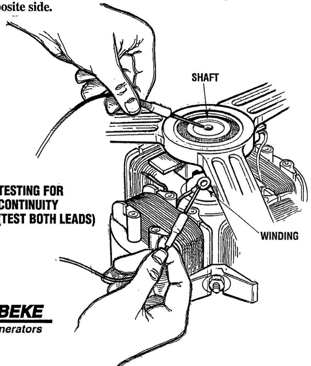
TESTING FOR CONTINUITY (TEST BOTH LEADS)
