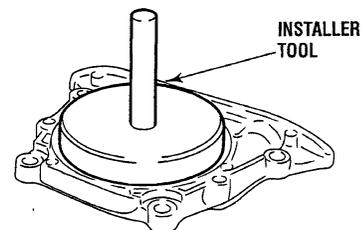
3. Install the oil seal case into the cylinder block through the gasket. (If there is no gasket, coat with sealant.) The entire circumference of the oil seal lip should be coated with clean engine oil.
