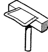
**CRANKSHAFT REAR OIL SEAL INSTALLER**
