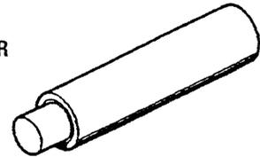
**PIN** *For supporting the sprocket when the camshaft sprocket is loosened or tightened.*
