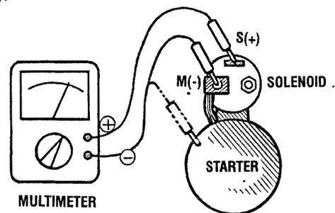
**NOTE:** Disconnect the wire from terminal M.
