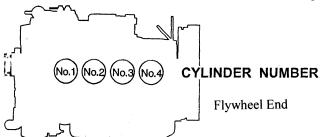
The sequence of cylinder numbers is given as No.1, No.2, No.3 and No.4 starting from the gear case side.
