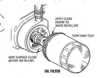
3. Filling the Oil Sump. Add new oil through the oil filler cap on the top of the engine or through the side oil fill. After refilling, run the generator for a few moments while checking the oil pressure. Make sure there is no leakage around the new oil filter or from the oil drain system, and stop the engine. Then check the quantity of oil with the lube oil dipstick. Fill to, but not over the high mark on the dipstick, should the engine require additional oil.
