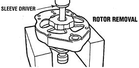
**NOTE:** If the bearing is removed from the housing, a new bearing must be installed.
