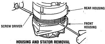
14. Carefully push the rotor assembly out of the front housing and rear housing.
