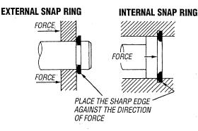
When reassembling external or internal snap rings, position them so that the sharp edge faces against the direction from which force is applied.
