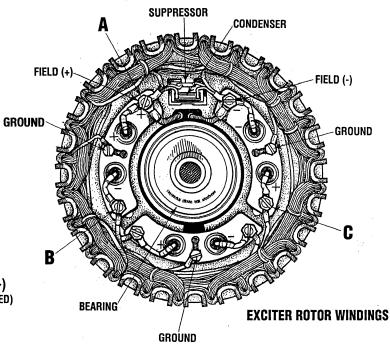
Disconnect these three wires from the diode bridge plates taking care not to drop any screws or washers.
