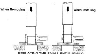
REPLACING THE SMALL END BUSHING
