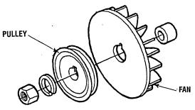
**PULLEY AND FAN COMPONENTS**
