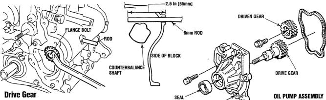
Align the timing marks and install the oil pump drive gear to the cylinder block.
