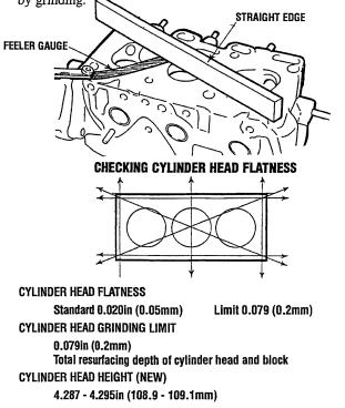
**CAUTION:** No more than 0.079in (0.2mm) of stock may be removed from the cylinder head and cylinder block mating surfaces in total.
