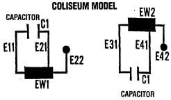
MAIN STATOR WINDING RESISTANCE LESS THAN ONE OHM FOR EACH WINDING GROUP
