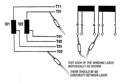
No Continuity between Isolated Stator Windings and Ground
