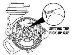
Adjust the point gap of the pick-up assembly between the rotor and the pick-up.
