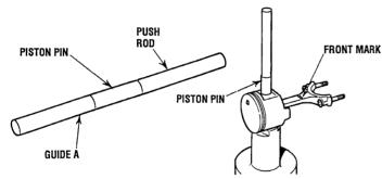
Set up the piston and connecting rod on the piston pin setting base. Make sure that the front marks are facing up. Apply engine oil to the outer circumference of the piston pin and insert the pin, Guide A and the push rod (assembled) into the piston and connecting rod.
