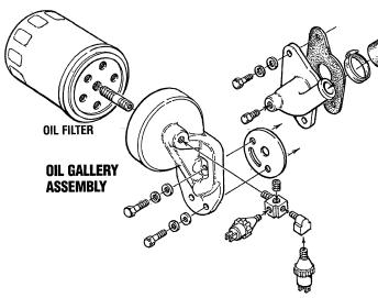
Disconnect and drain the oil hoses. remove, clean and inspect the oil gallery/filter assembly, replace the filter.
