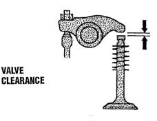
Valve Clearance: INTAKE EXHAUST
