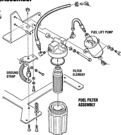
Remove the fuel filter assembly. Drain and inspect the hoses. Inspect the O-ring and replace the filter element.
