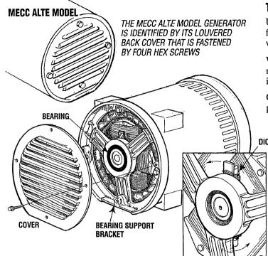
Testing the Mecc Alte generator can be accomplished without removing the bearing support bracket. Simply turn the armature to allow access for the testing as shown.
