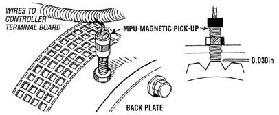
**NOTE:** If replacing the Magnetic Pick-Up (MPU) it **MUST** be replaced without cutting and splicing into the existing wiring cable. Doing so will cause a erratic AC signal to the controller.
