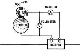
A CAUTION: Use thick wires as much as possible and tighten every terminal securely. This is a solenoid shifttype starter which makes a rotating sound louder than that of a direct-drive type starter. When detecting starter rotation at the pinion tip, be careful not to come in contact with the pinion gear when it protrudes.
