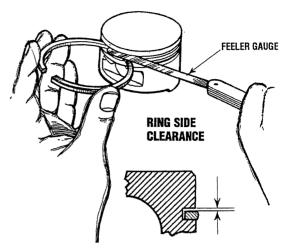
Check the clearance between the piston ring and the ring groove, if it exceeds the limit, replace the rings, the piston or both.
