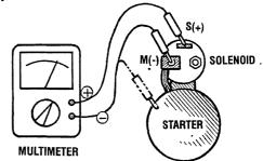
**NOTE:** Disconnect the wire from terminal M.
