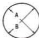
MEASURING MAIN BEARING I.D.
