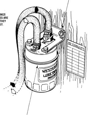
APPLY A THIN COAT OF CLEAN OIL TO THE FILTER GASKET WHEN INSTALLING. AFTER THE FILTER CONTACTS THE BASE, TIGHTEN IT AN ADDITIONAL 3/4 TURN.
