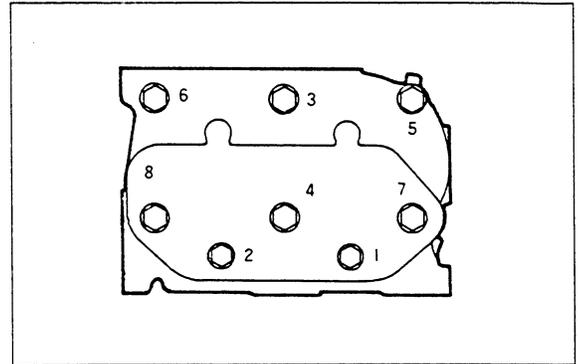
Cylinder Head Bolt Tightening Sequence
