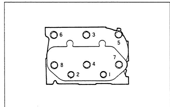
Sequence for Tightening Cylinder Head Bolts
