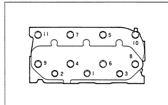
Sequence for Tightening Cylinder Head Bolts
