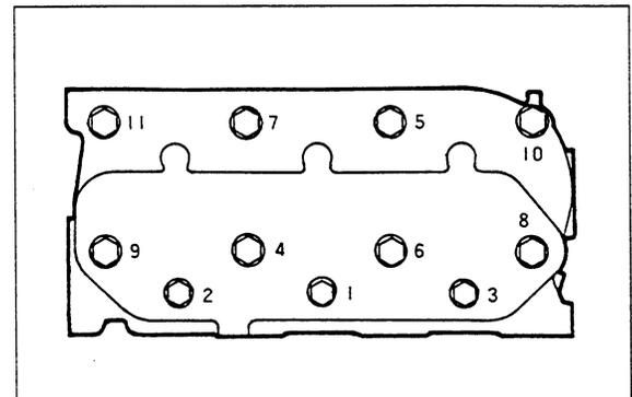
Cylinder Head Bolt Tightening Sequence
