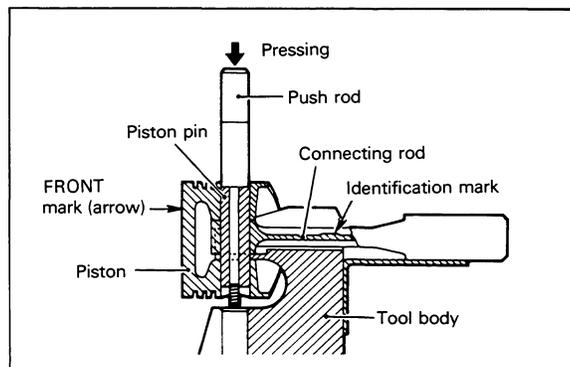
Installation of Piston and Connecting Rod
