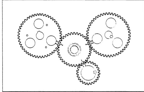
Timing Gears in Alignment with Each Other
