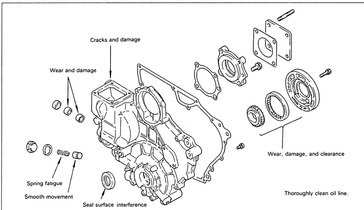
Inspection of Gear Case and Oil Pump
