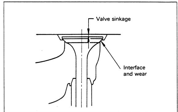
Checking Valve Sinkage
