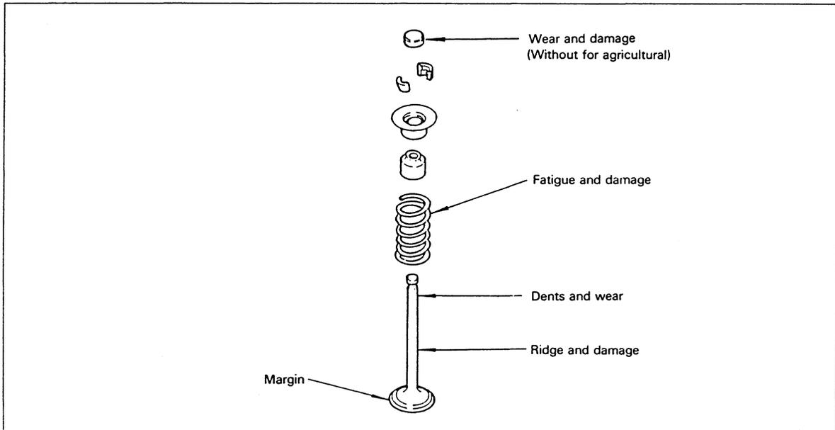
Inspection of Valve and Valve Spring
