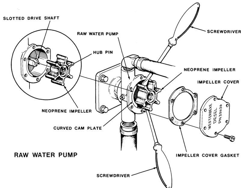
Remove the impeller with the aid of two small screwdrivers, as illustrated, and carefully pry the impeller out of the pump. Install the impeller by positioning the hub pin to align with the slot in the drive shaft. Move the blades to conform to the curved cam plate and push the impeller into the pump's housing.
